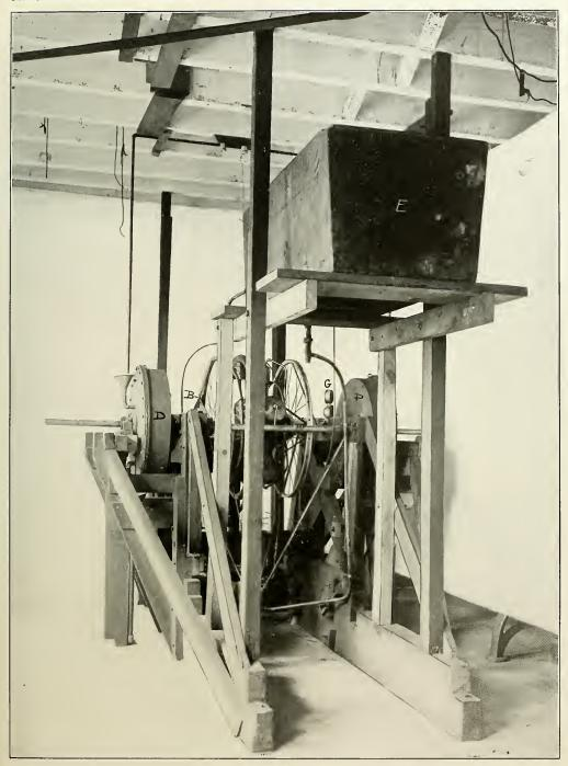
DYNAMOMETER TESTS OF LARGE ENGINE
